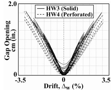
**Figure 6. Gap opening along base joint at wall centerline.**
