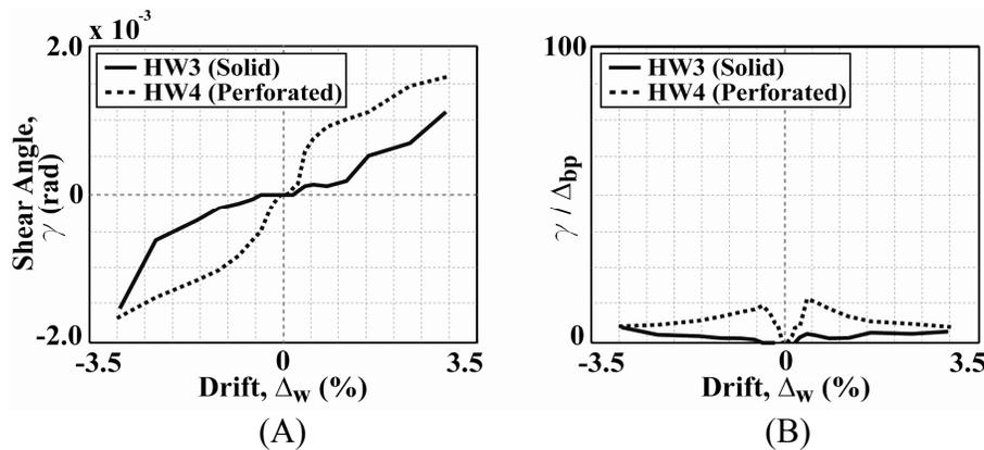
**Figure 7. Shear deformations of base panel: (a) shear distortion angle; (b) shear distortion angle normalized by total base panel drift.**
