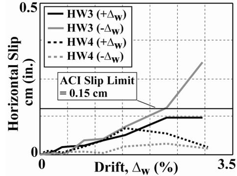
**Figure 8. Horizontal slip along base joint.**
