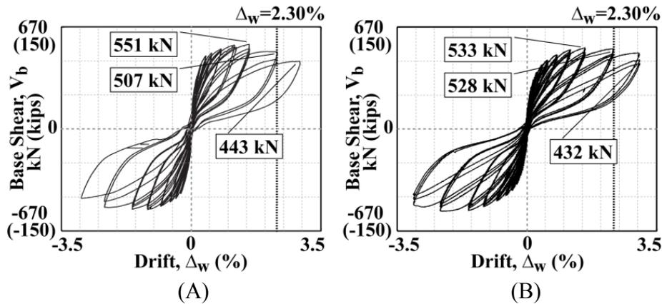
**Figure 4. Base shear force versus wall drift history:**
