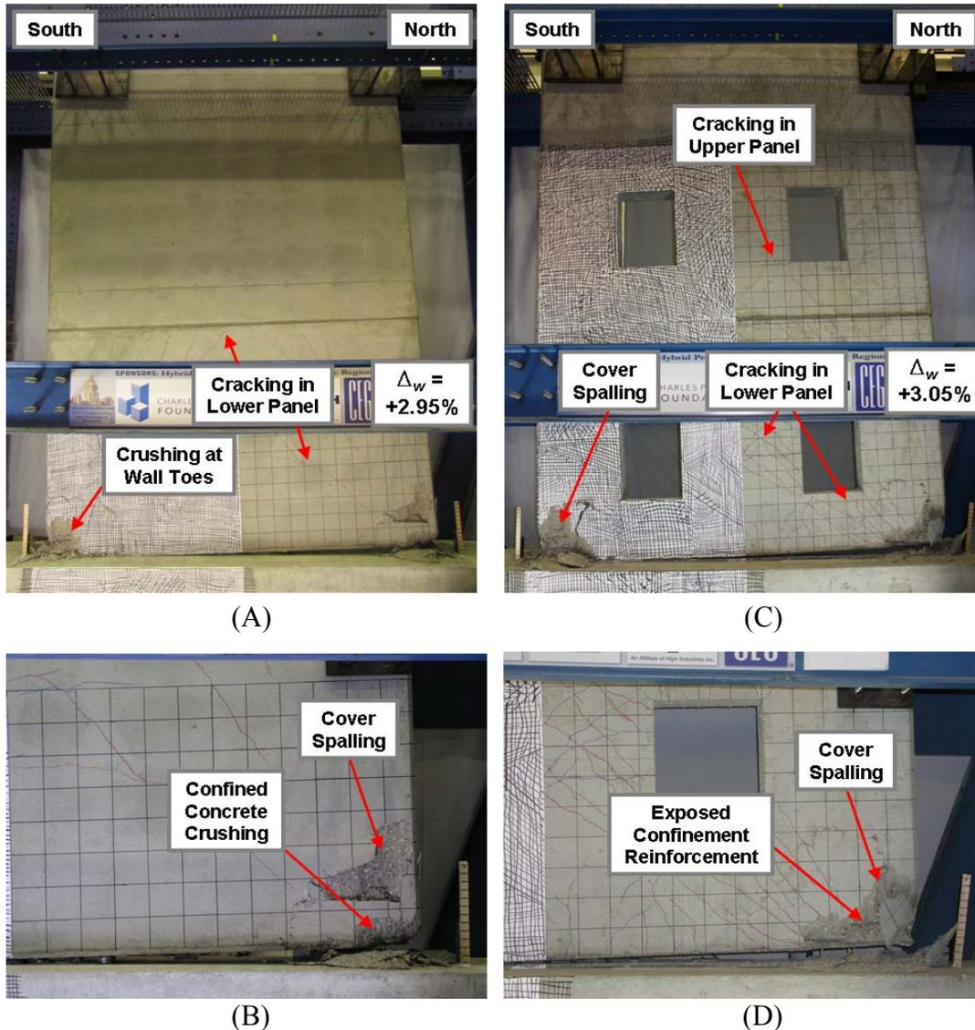
**Figure 3. Observed damage: (a) HW3 at third cycle of  $\Delta_w = +2.95\%$ ; (b) north end of HW3; (c) HW4 at third cycle of  $\Delta_w = +3.05\%$ ; (d) north end of HW4.**
