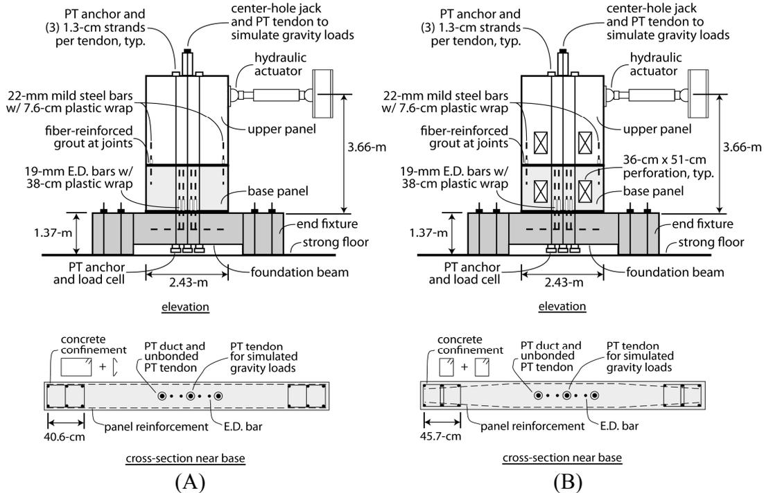
**Figure 1. Test configuration and specimen details:**
