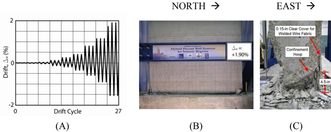
Figure 3. Wall Behavior: (a) Applied Displacement History; (b) Damage at Third Cycle of  $\Delta_w=+1.90\%$ ; (c) South Toe of Wall after Completion of Test
