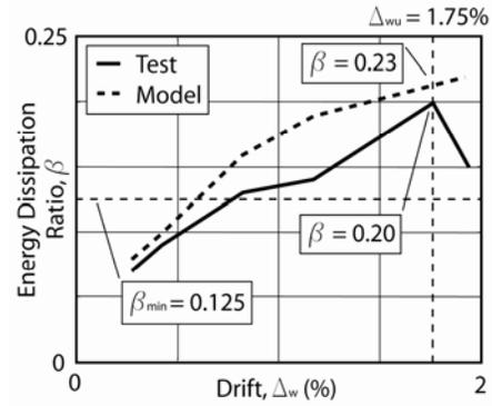
Figure 6. Energy Dissipation Ratio
