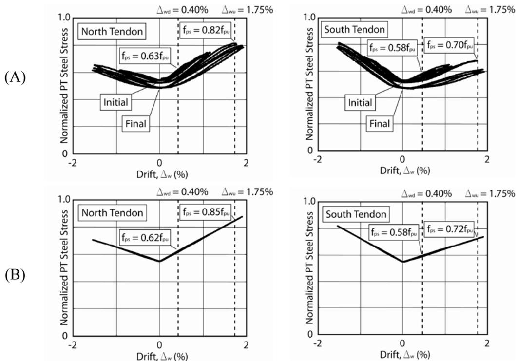
Figure 9. Average PT Steel Stresses: (a) Measured; (b) Analytical
