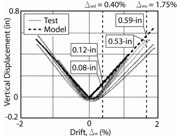
Figure 11. Vertical Displacements at Wall Top
