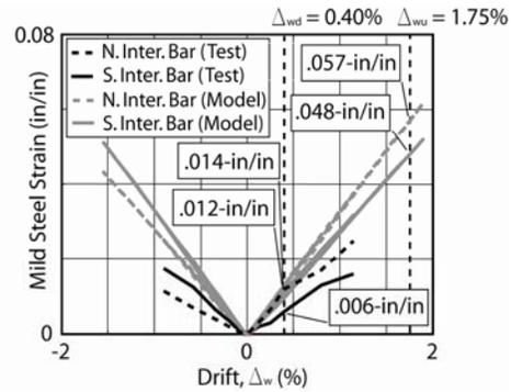
Figure 8. Measured and Analytical Strains in North and South Intermediate Mild Steel Bars
