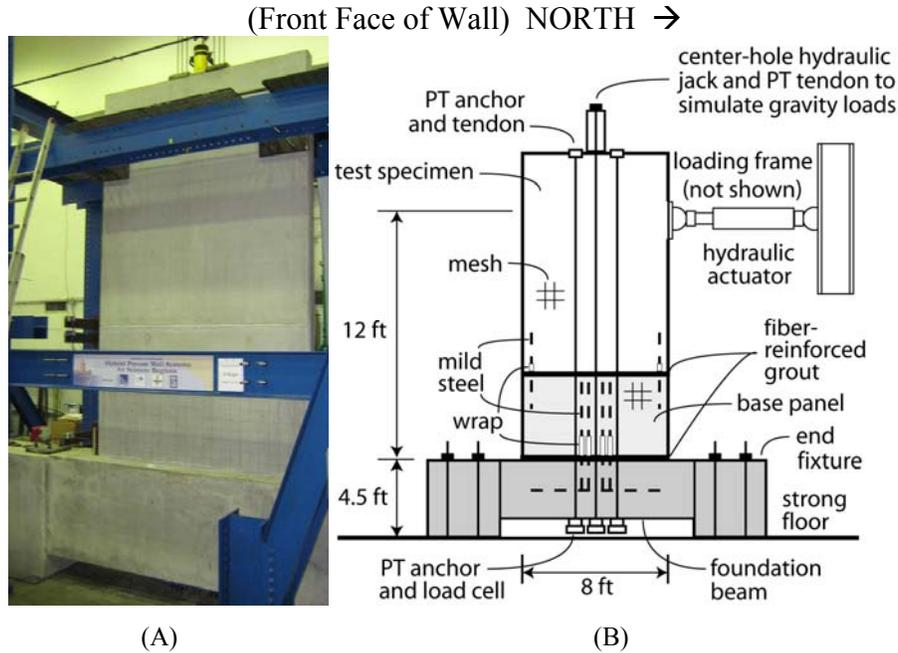
Figure 2. Test Set-Up: (a) Photograph; (b) Schematic Drawing
