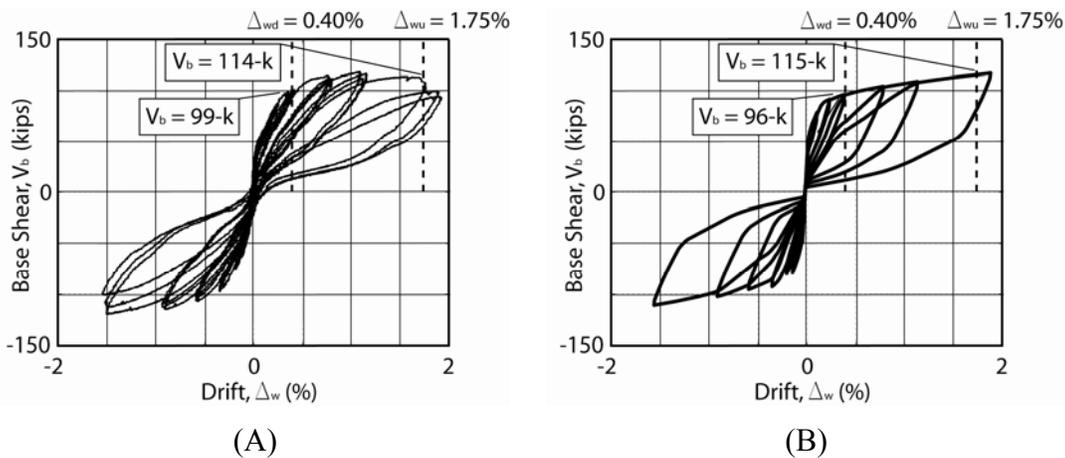
Figure 5.  $V_b/\Delta_w$  Behavior: (a) Measured; (b) Analytical
