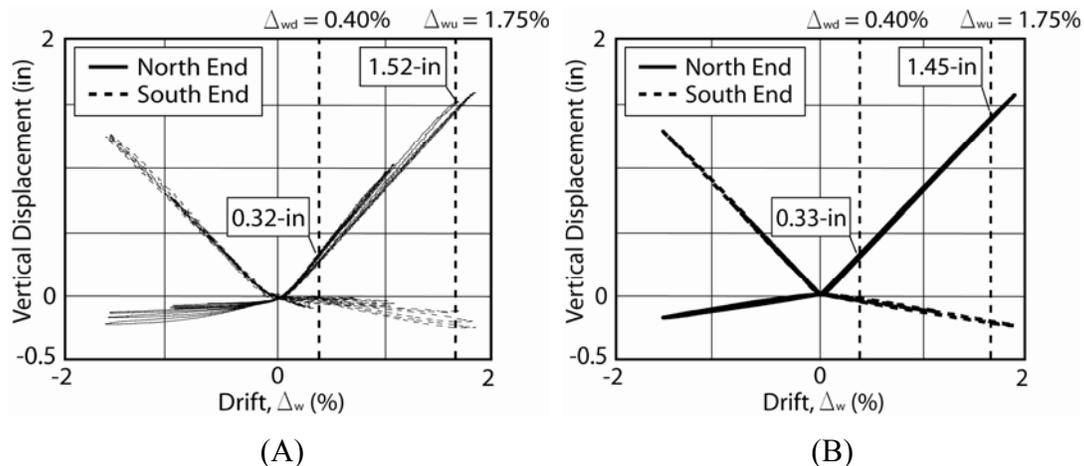
Figure 10. Vertical Gap Opening Displacement at Wall Toes: (a) Measured; (b) Analytical
