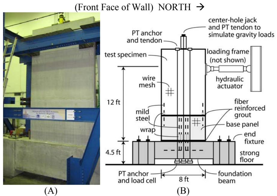
Figure 3. Test Set-Up: (a) Photograph; (b) Schematic Drawing
