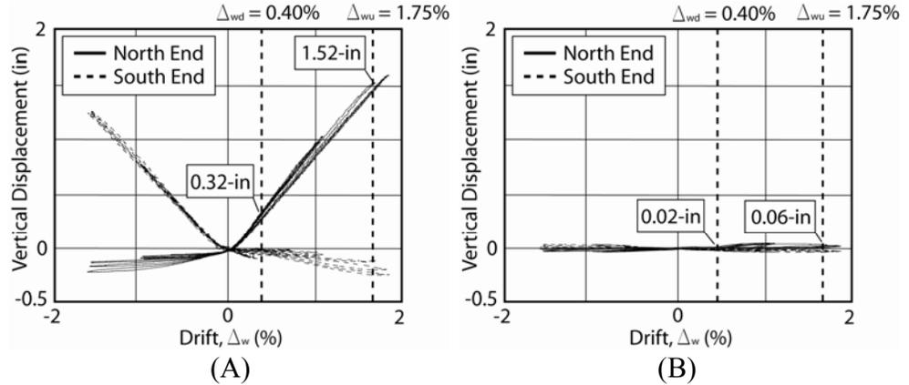
Figure 9. Vertical Gap Opening Displacement at Wall Ends:
