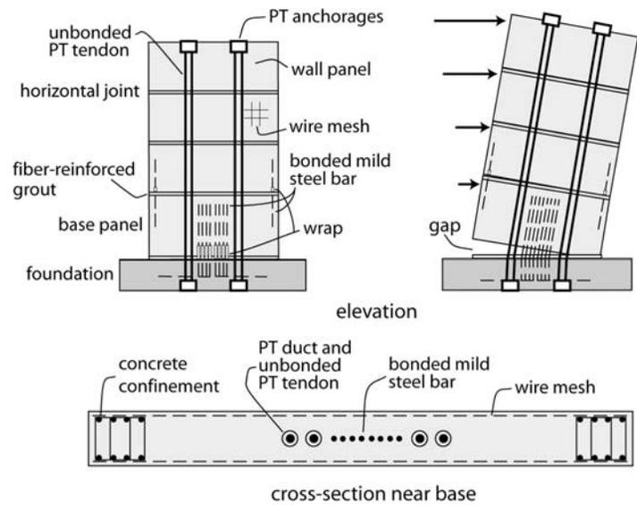
Figure 1. Elevation, Exaggerated Displaced Position, and Cross-Section of Hybrid Wall System
